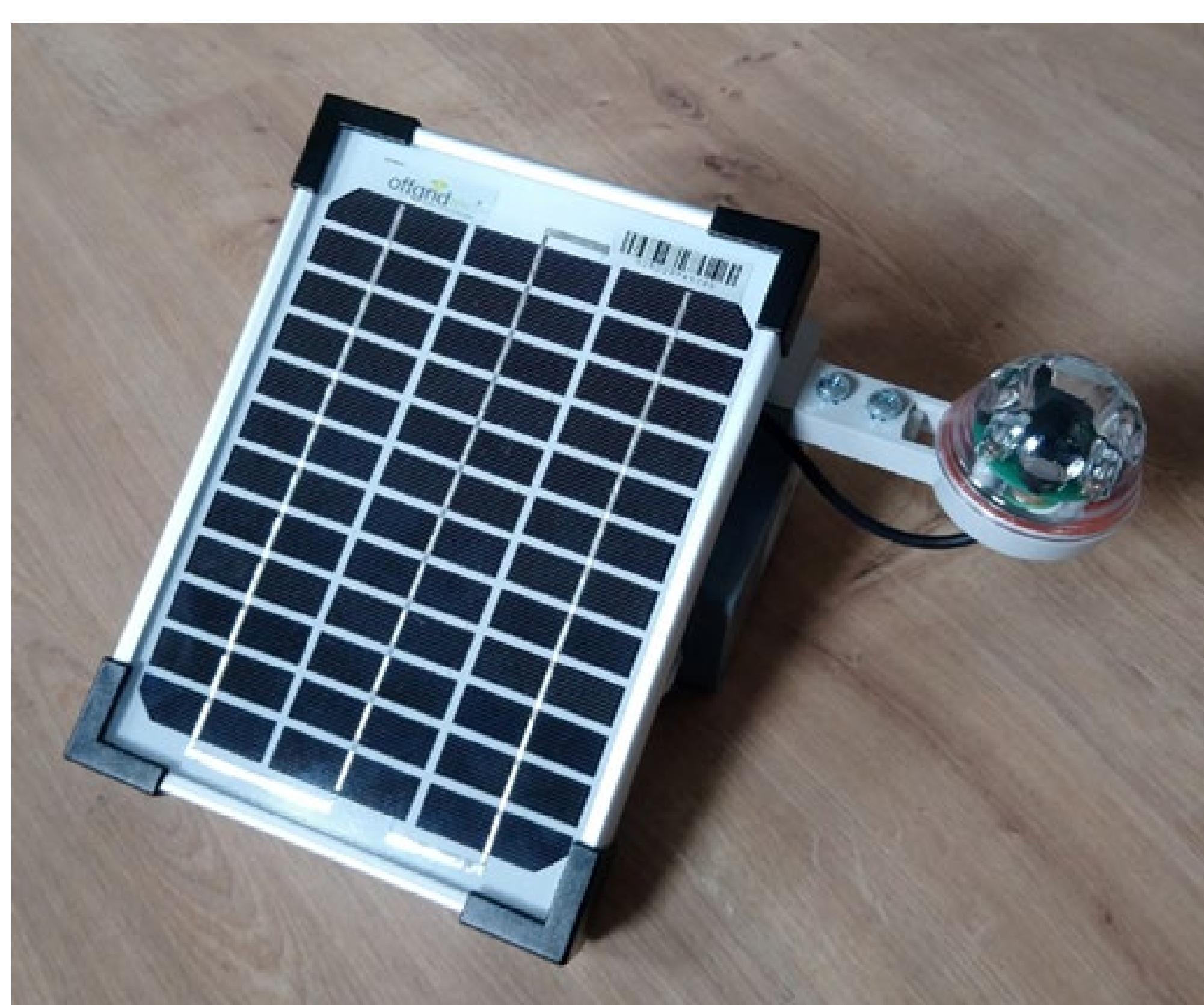
Figure 1 – This is one of the optical IoT IR sensors
